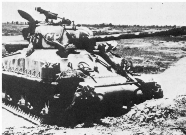
An M4A1 (76mm, Remanufactured) lurks in hull defilade during the fighting in Kashmir. This vehicle, believed to be of the Pakistani 26th Cav. Regt., is armed with the 76mm M1 tank gun fitted in the older, smaller 75mm turret. During the 1965 war both the Pakistanis and the
