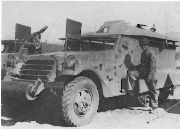
While Maj.Gen. George S. Patton commanded the 1st Armored Corps at the Desert Training Center in the US in 1942, he used this 'customised' M3 command half-track. This vehicle is shown as Plate A1, as it appeared after its insignia had been added.
