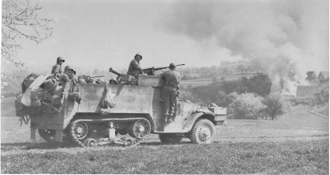
A light machine gun squad of the 61st Armd. Inf. Bn. move forward through the German countryside on 17 April 1945. The half-track would appear to be an older M3 (winch) which has been rebuilt with an M49 ring mount and pulpit. Newly manufactured M3A1s had mine racks fitted to the hull side, which this vehicle, like many M3s, lacks. The half-track's armament includes both an air-cooled and a water-cooled .30cal. Browning. (US Signal Corps)
