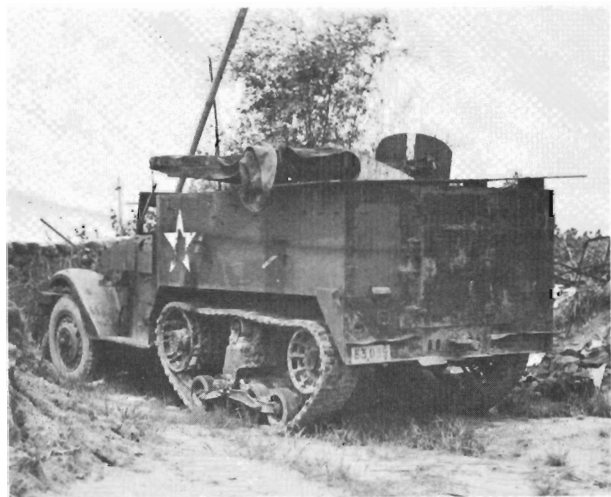
Small numbers of half-tracks left over by the French were used by the South Vietnamese during the Vietnam War, like this M3 of the 1st ARVN Cav. Regt. sitting behind a protective berm. It is armed with M2 .50cal. and .30cal. machine guns behind improvised armour shields. (James Loop)
