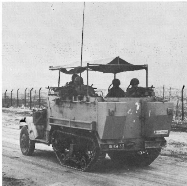
The most prominent user of half-tracks after 1945 was the Israeli Army. They formed the backbone of the Zahal armoured infantry, only beginning to be replaced at the time of the 1973 war. They still remain in service in various rôles like this rebuilt M2 being used for border patrol. Like most of the rebuilt half-tracks, it has added rear fuel tanks besides automotive improvements such as the 6V53 diesel engine. (IDF)
