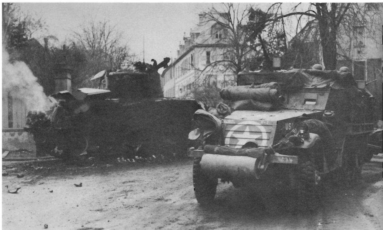
An M3A1 of an infantry anti-tank squad of the 14th Arm. Div. passes the burned-out wreck of an M4A3(76mm)W knocked out the previous evening, 28 November 1944, by Tiger tanks during the fighting for Barre, France. Besides the prominent Allied star, the vehicle's name 'Baby Bastard No. 1' can be seen on the armoured radiator cover. (US Signal Corps)
