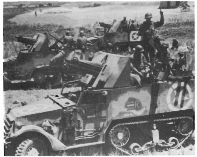
T30s of the US 2nd Armd. Div. take up firing positions near Licata, Sicily, during the fighting in 1943. Besides their main armament these vehicles each have a pair of .30cal. machine guns added on improvised mounts. They are camouflaged in a pattern of Olive Drab and Sand, common to most 2nd Armd. Div. vehicles on Sicily. The use of the circled star was first mandated for the Sicily operation to prevent inadvertent Allied air attack.
