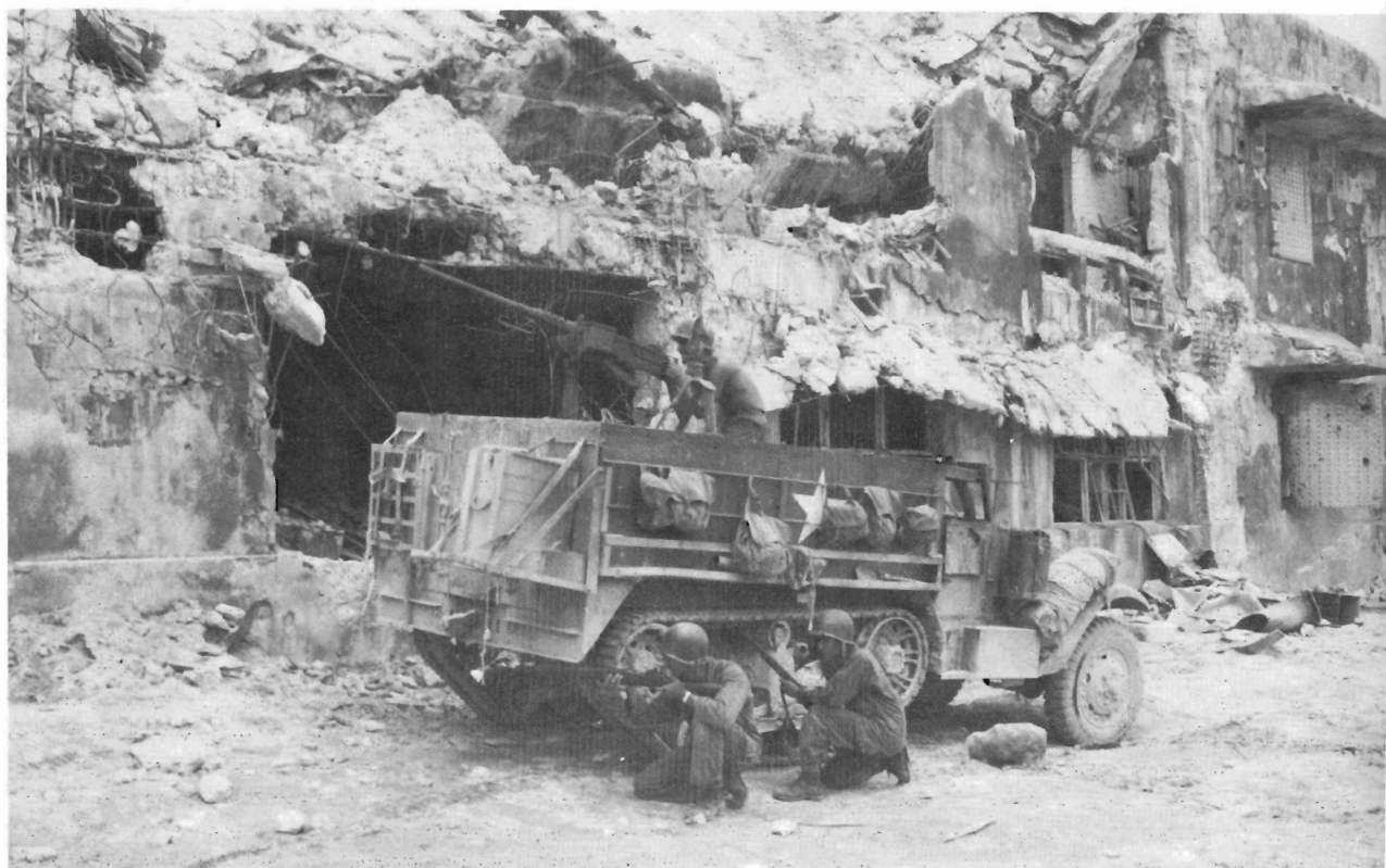
The personnel carrier version of the M3 half-track was not particularly common in the Pacific, its use being confined mainly to headquarters and maintenance units. This HQ vehicle took part in the fighting near a wrecked plant on Peleliu, Caroline Islands, in 1944. (US Signal Corps)
