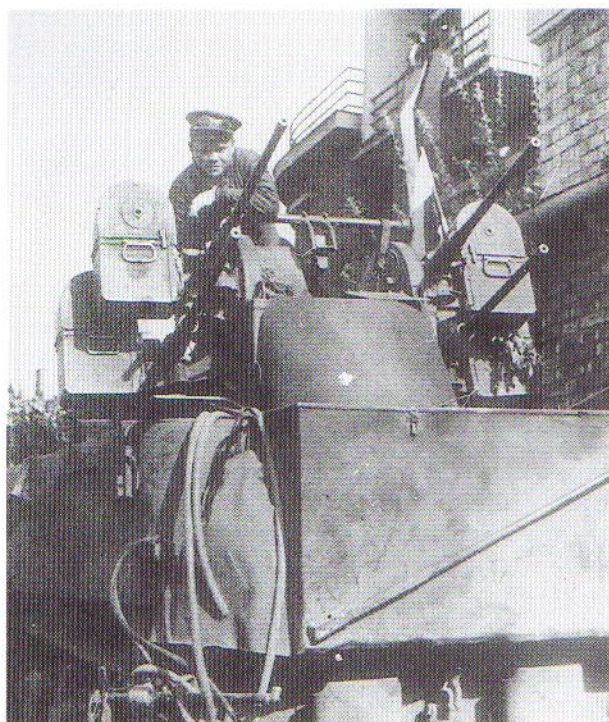
The M17 was the International Harvester equivalent of the M16 MGMC, but based on the M5 half-track instead of the M3. Like this example
