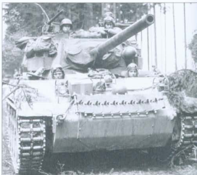
A M18 tank destroyer with the 602nd Tank Destroyer Battalion supporting the 89th Division during operations in the Lossnit forest in May 1945. The crew has mounted an additional .30-cal. machine gun on the right side of the turret near the loader typical of efforts to improve the self-defense capability of these vehicles. The use of BAR automatic rifles for close-in defense was popular in some units. (NARA)
