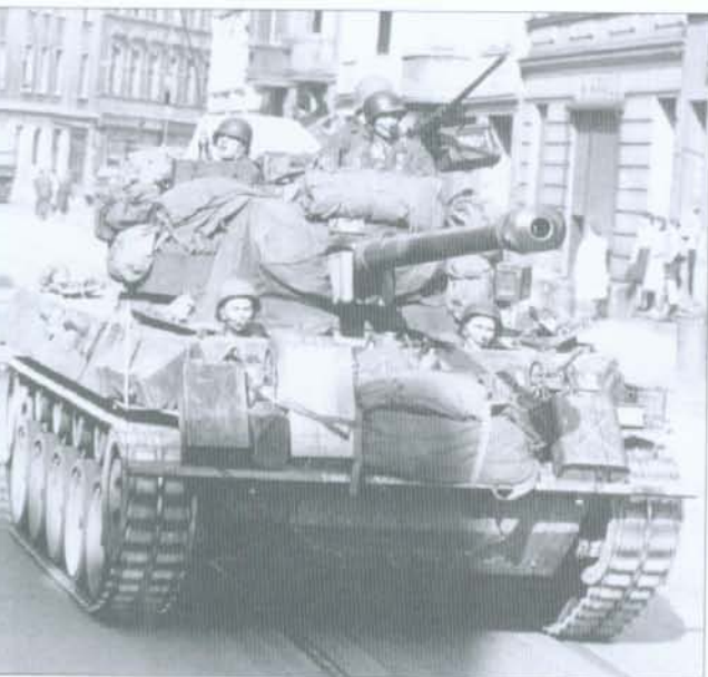
This is another example of a late production M18 with muzzle brake in service in Germany in April 1945, this time passing through Dusseldorf. This unit has attached a plank along the front to carry additional stowage. (ARA)
