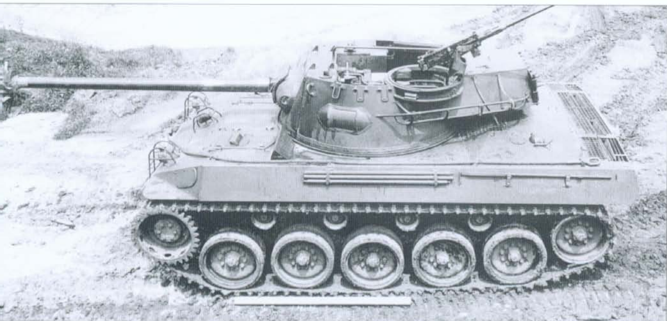
The T70 76mm GMC was configured from the T67 with the transmission in front and the addition of a bustle to the turret. This is the third pilot during trials at Aberdeen Proving Ground in 1943. (Patton Museum)
