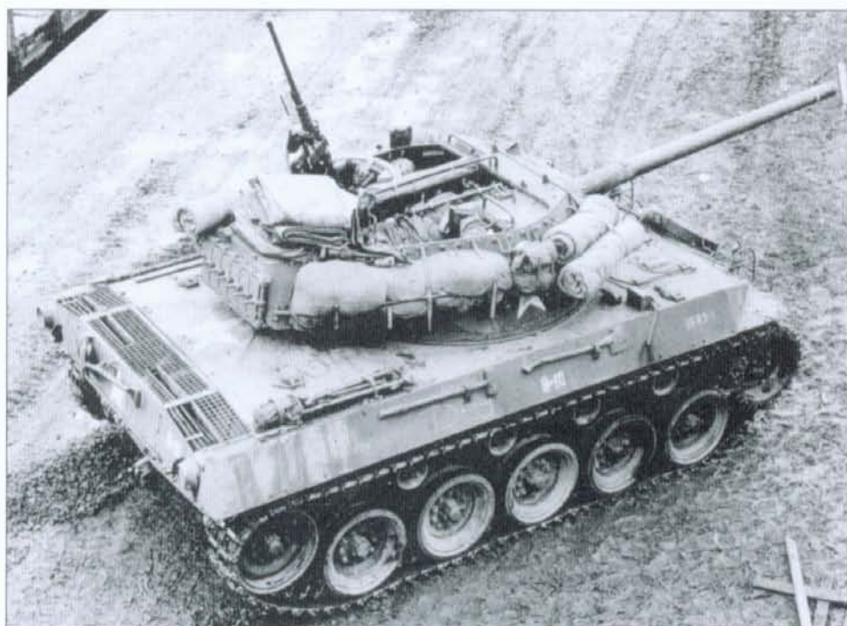
The M18 76mm GMC was viewed by the Tank Destroyer command as the ideal tank destroyer of the war. This is a GMC of Co. B, 827th Tank Destroyer Battalion, manufactured in the initial contract run in December 1943 and is fairly typical of the M18 tank destroyers that saw combat in France in the summer of 1944. (NARA)
