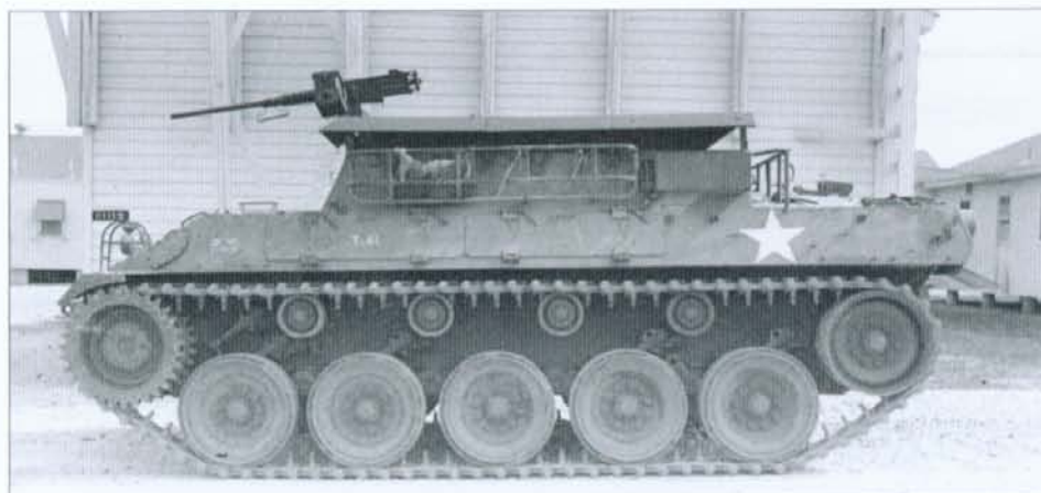
The vulnerability of the open troop compartment in the M39 AUV led to experiments with one of the T41 pilots at Fort Knox. A simple roof was added over the hull opening, but this was not accepted for production. (Patton Museum)
