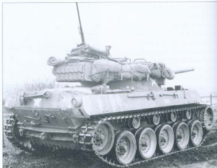
This is a good example of a production M18 76mm GMC manufactured in December 1943 from the original contract batch of 1,000 vehicles. It is seen here serving with Co. B, 827th Tank Destroyer Battalion. The extensive external crew stowage was necessary since so little could be carried inside the cramped hull interior. This is typical of service vehicles which often had the fragile front and rear mudguard removed due to their tendency to get in the way during routine track maintenance. (NARA)
