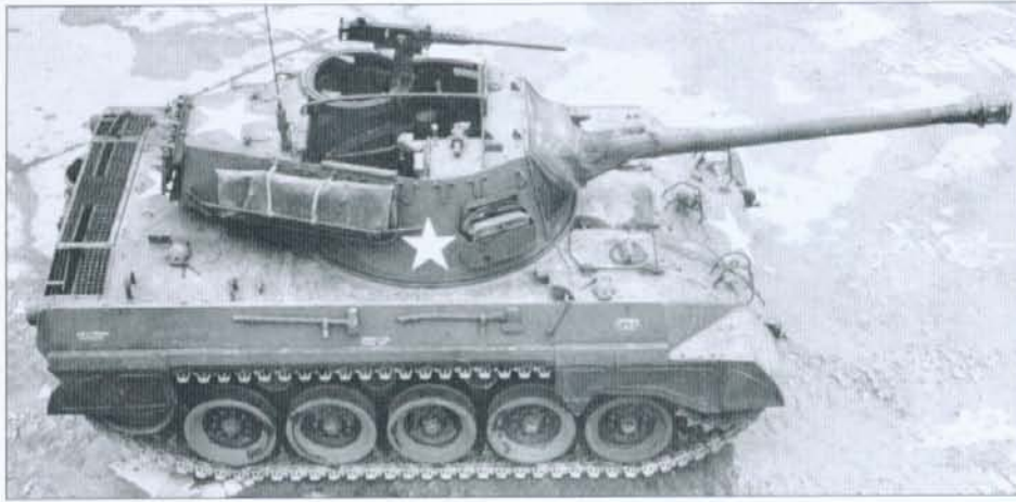
This is M18 serial 2507 (registration number 40146389), the last M18 manufactured in October 1944. It shows the final configuration of the vehicle including the wider 21-in. tracks and the additional dust-guard running along the length of the hull. This also shows the official stowage, including the drivers' foul weather hood stowed in the special rectangular pannier on the front of the turret. (MHI)
