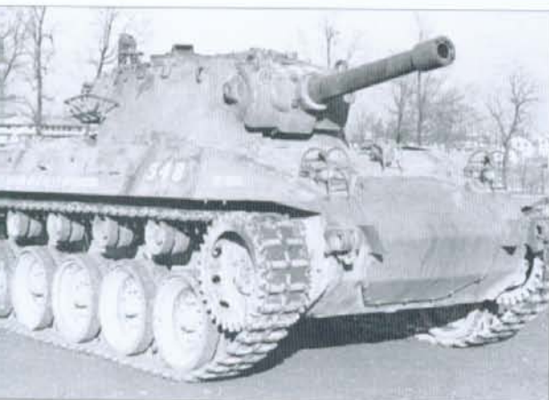
The T88 105mm HMC was an attempt to develop a more satisfactory assault gun for cavalry units than the existing M3 75mm HMC on the M5A1 tank chassis. This shows one of the T88 pilots at Fort Knox during trials in early 1945. The program ended before the type could be put into production. This particular vehicle has been modified with adapter plates on the bow to permit attachment of the Ritchie T7 device. (Patton Museum)
