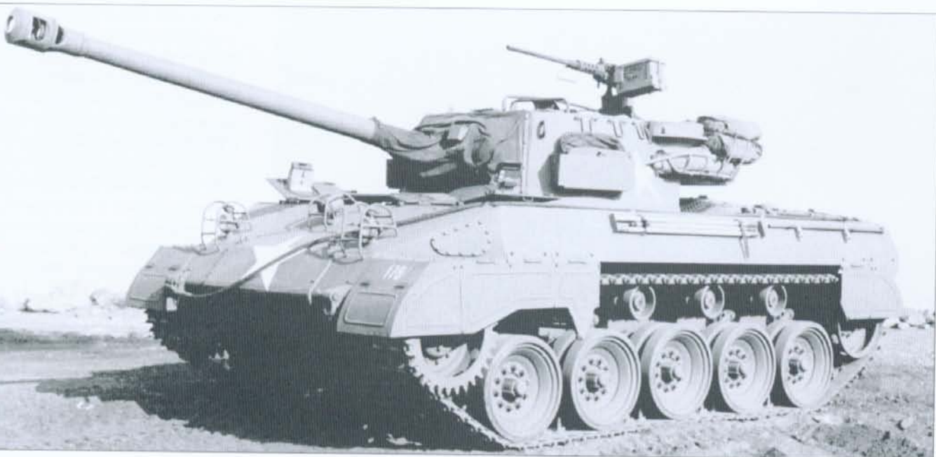
late production M18 76mm GMC, accepted in September 1944. Roughly the last 700 of the M18 were fitted with the M1A2 76mm gun and muzzle brake as seen here. This also provides a good view of the standard mudguards, a feature seldom seen on vehicles in combat. (Patton Museum)
