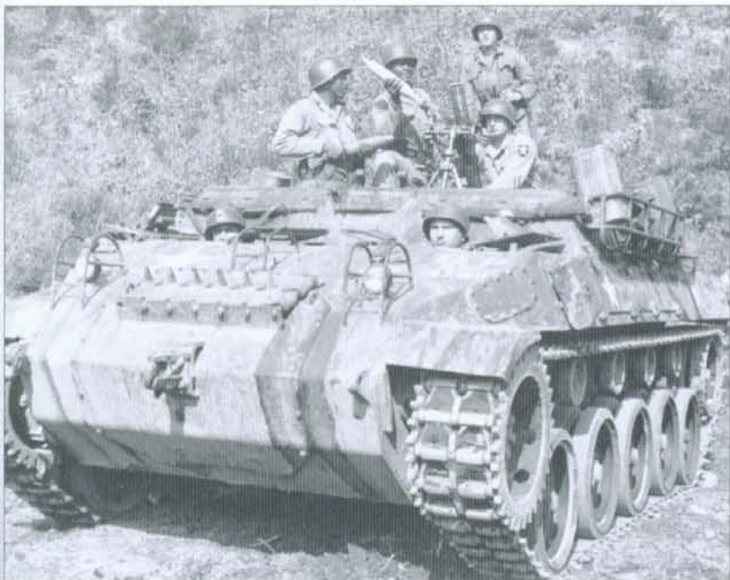
The 72nd Tank Battalion, 2nd Infantry Division converted some of their M39 AUVs into self-propelled 81mm mortar vehicles seen here in action in Korea on March 21 1952. (NARA)
