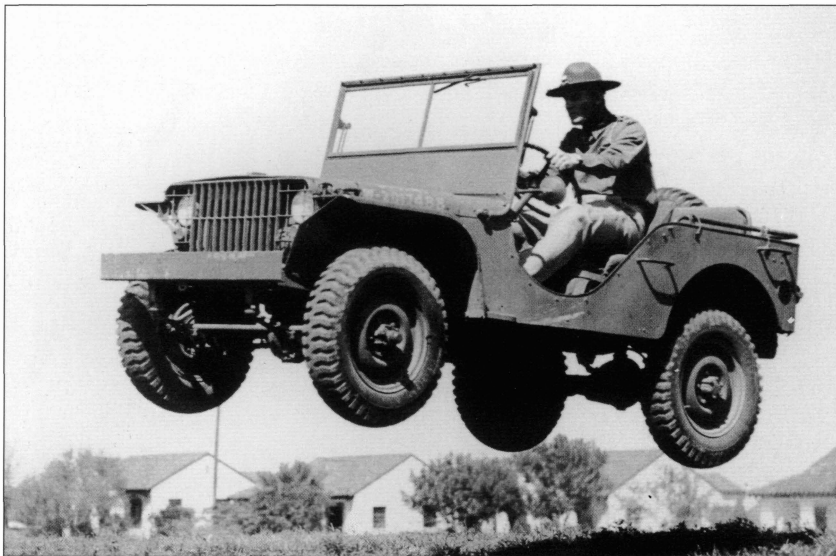
The Ford GP shows close similarities to the standardized jeep but can be distinguished by its slat grill. This is the 67th production vehicle from the original contract and is seen here during tests at Fort Sam Houston in April 1941.
