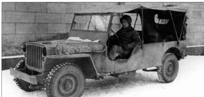
Some US units lengthened jeeps in the field to provide more passenger space in the rear. This is one from the 127th Ordnance Maintenance Battalion in Belgium on January 23, 1945. (NARA)
