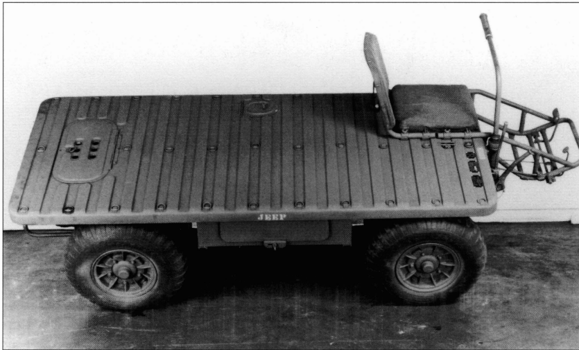
The final wartime attempt at a lightweight jeep was also the most futuristic, the Willys JBC Jungle Burden Carrier. Although too late to enter production, it pioneered the way for similar vehicles after the war, such as the M274 1/2-ton 4x4 Mechanical Mule. (USAOM-APG)
