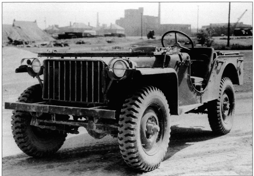
The Bantam 40 BRC began to take on the more distinctive look of the wartime ¼-ton trucks with its new slat grill. It can be distinguished from the Ford GP and Willys MA by the recessed mount for the headlights on the front fenders. (NARA)
