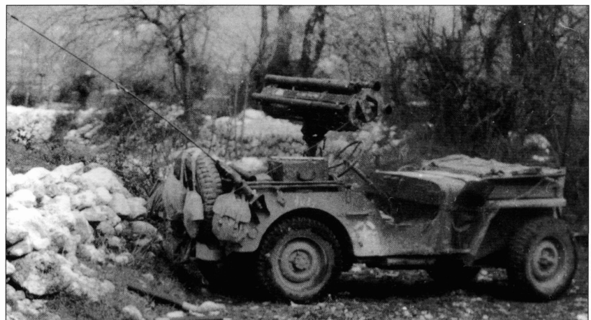
There were numerous attempts to arm jeeps with the 2.36in bazooka antitank rocket launcher. This jeep, along the Rapido river in Italy in January 1944, has been fitted with an improvised frame mounting to mount at least four bazookas for some salvo firepower. (NARA)
