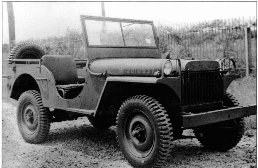
The Willys MA introduced a reconfigured body with a slat grill, but distinguishable from the later MB by the truncated hood with Willys logo and fender-mounted headlights. (MHI)
