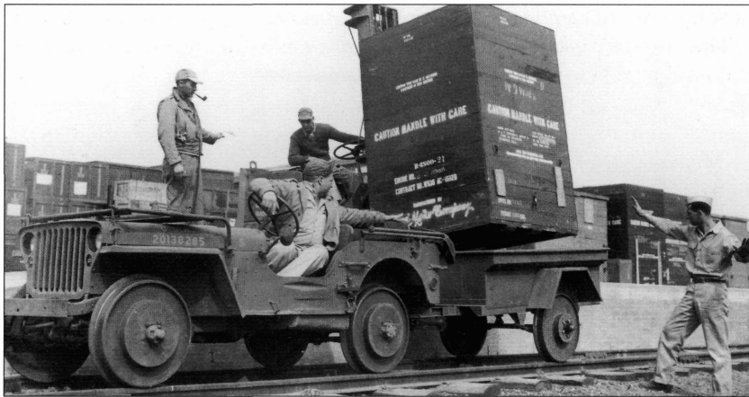
The jeep was often adapted to run on rails, using both kits and local improvisations. This Ford GPW produced in August 1942 is seen being used as a rail tug in Australia in August 1943, with the standard 1ton trailer also being adapted for use on rails. (NARA)
