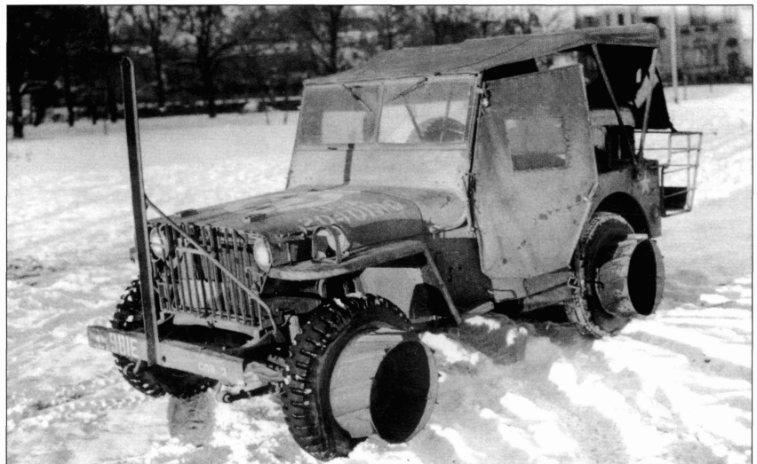
There were a number of attempts to improve jeep performance in the snow, including several configurations of drums added at the wheel to decrease ground pressure in deep snow, as seen on this early production Willys MB slat grill of the 981st Engineer Maintenance Company in Belgium on January 15, 1945. This jeep has several other common field modifications, including the common antiwire device on the bumper and a stowage bin added at the rear. (NARA)
