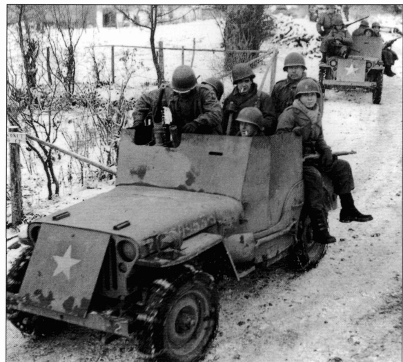
The 82d Airborne Division developed its own standardized armor kit for its recon jeeps, as seen here during the Battle of the Bulge in January 1945.
