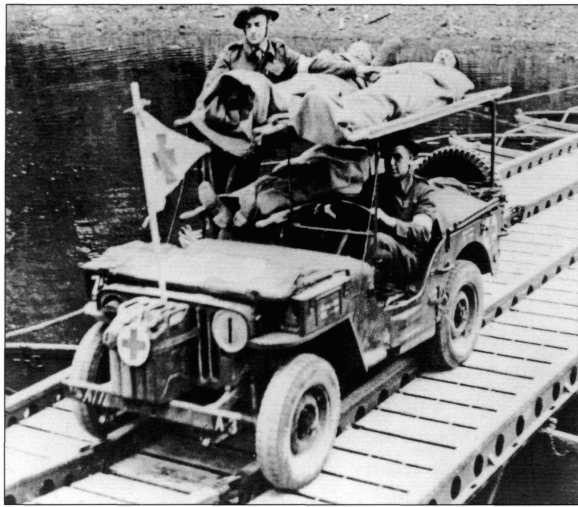
The British ambulance configuration used a frame to hold the litters over the top of the jeep, like this one, crossing a tactical bridge near Caen in late July 1944. (NARA)
