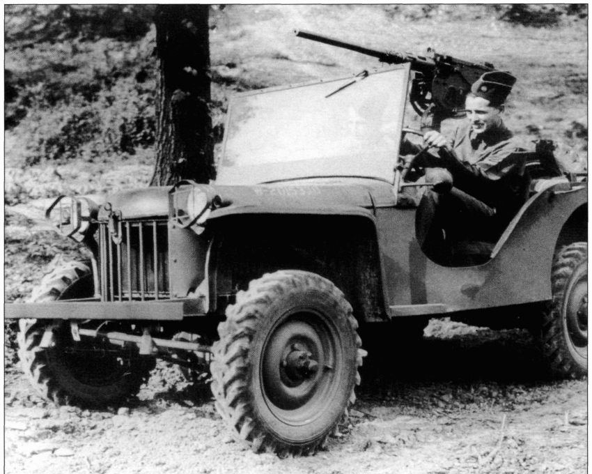
This Bantam Mark II is the sixth production vehicle from the original contract and is seen here on maneuvers with the 1st Armored Division at Fort Knox in 1941, armed with a Browning .50-cal. heavy machine gun. The Bantam was easily distinguishable from later ½-ton trucks by its round front hood. (MHI)
