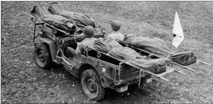
Jeeps were widely used as field ambulances, but their small size led to improvisations to carry the litters. This October 1943 Ford GPW from the 6th Armored Division in England in June 1944 shows the addition of simple frames to permit the carriage of four litters. (NARA)
