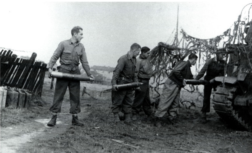
Below: Men of 2nd Armored load 105mm shells onto an M7 HMC, on October 25, 1944, just after the fall of Aachen. The standard weapon of the armored division's artillery units, the M7 HMC had the chassis of the M3 medium, the M7B1 that of the M4. The main armament was a 105mm M1A2, M2 or M2A1 howitzer fired by a gun crew of five, bringing the total crew to seven including commander and driver. U.S. Army via Real War Photos
