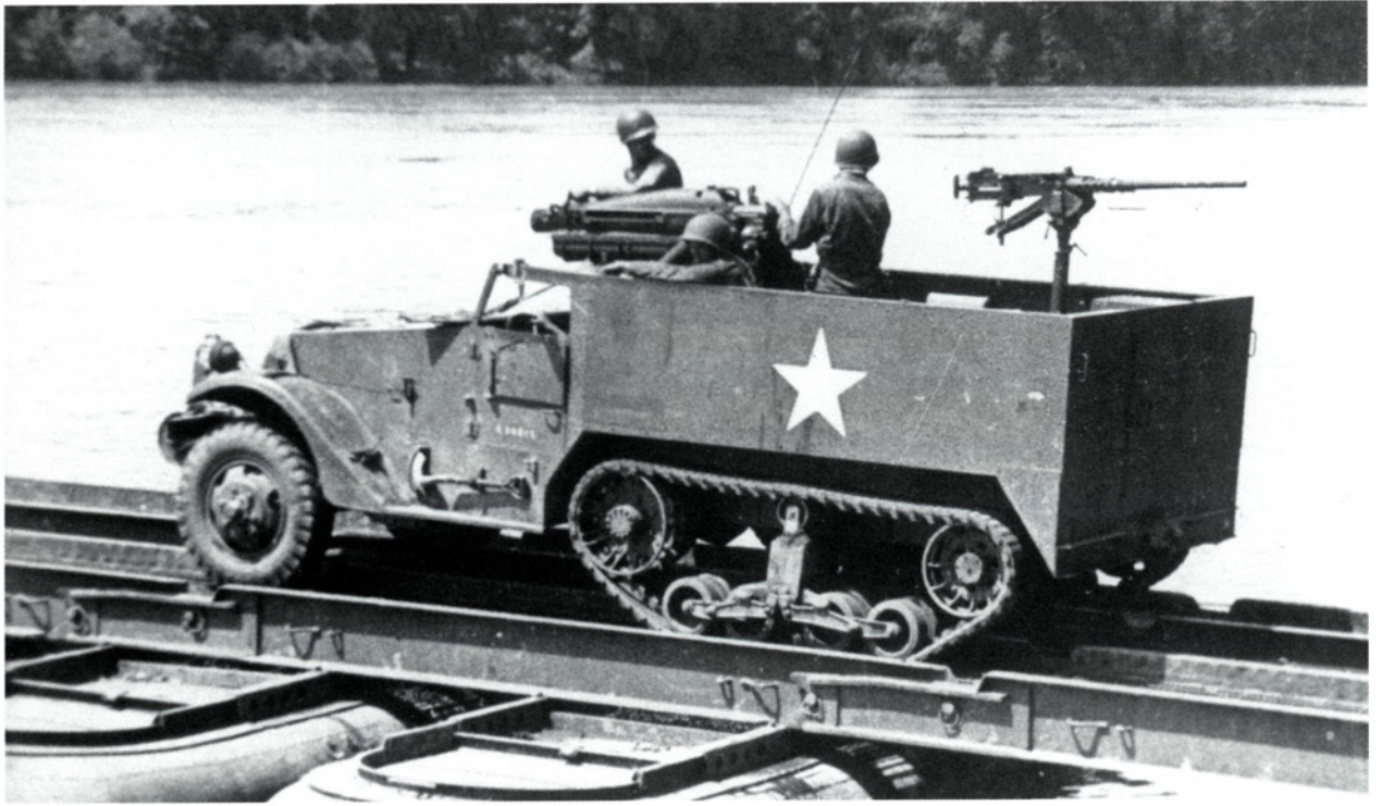
Above: The 75mm T30 howitzer motor carriage was used by HQ companies of medium tank battalions until replaced by the M8 HMC in 1943. This one carries a 75mm M1A1 howitzer and is seen at Fort Benning in July 1942. U.S. Army via Chris Ellis
