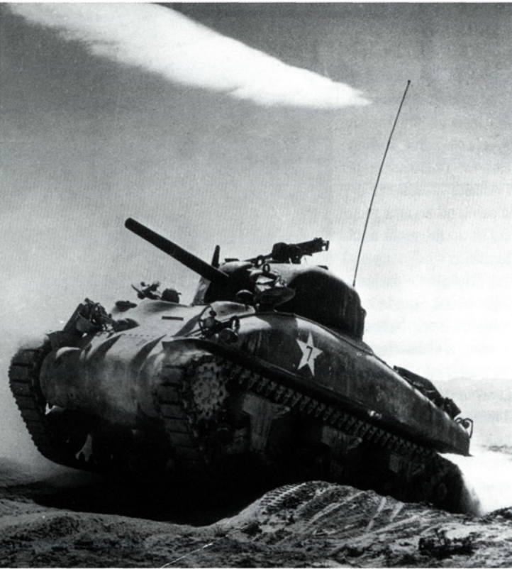
Above: A Sherman in action at El Guettar. Note the three-piece bolted nose section that identifies the early production vehicles; later production models had a one-piece cast hull. Via Chris Ellis
