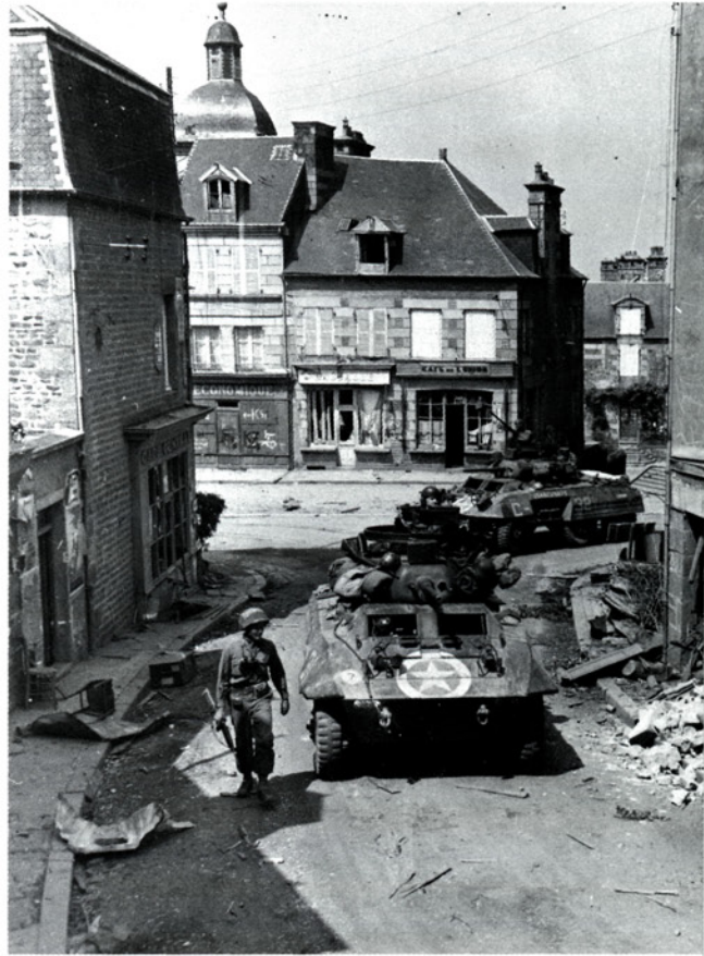
Above: Armored cars of the 82nd Reconnaissance Battalion wind through the streets of Calvados in Normandy on August 3, 1944. On its way to the town the 82nd had run into a bloody ambush in the forest of St. Sever. In picture are two M8 Greyhounds — wheeled armored cars that had a turret-mounted .50-cal MG and a crew of three.
