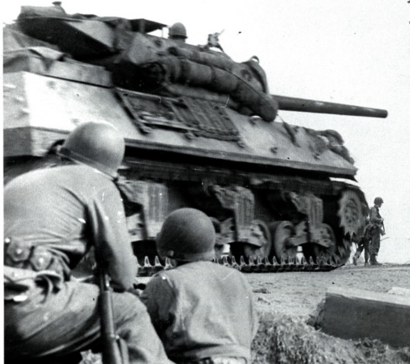
Left: The Gun Motor Carriages M10 (built on the M4A2 chassis) and M10A1 (built on the M4A3 chassis) equipped U.S. and British tank destroyer units. Over 6,000 were produced, around 1,000 being M10A1s which were mainly used for training or were converted into prime movers. In British service they were called Wolverines and from late 1944 many had the M7 3-inch gun replaced by 76mm OQF, being renamed Achilles. This M10 is seen outside Magdeburg on 17 April 1945 (see also pages 2/3). U.S. Army via Real War Photos
