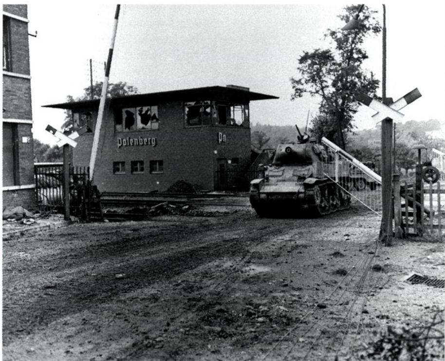
Above: An M8 assault gun of the 3rd Battalion, 67th Armored, moves past the railway station in Palenberg, Germany on October 4, 1944. At Palenberg, 2nd Armored established a bridgehead over the Wurm River on its first breach of the Westwall. The M8 was built on the chassis of the M5 light and provided a close-support howitzer that equipped HQ companies of medium tank battalions until replaced by the 105mm-equipped M4. Nearly 2,000 M8s were produced between the end of 1942 and January 1944.
