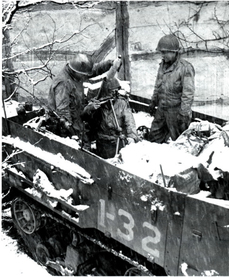
Above: In January 1945, during the Battle of the Bulge, 2nd Armored men operate their 81mm mortar from the rear of an M4A1 halftrack. A purpose-built mortar-carrying version of the M2, over 1,000 of the M4 and improved M4A1 (with strengthened floor to allow onboard use of mortar) versions were built. U.S. Army via Real War Photos
