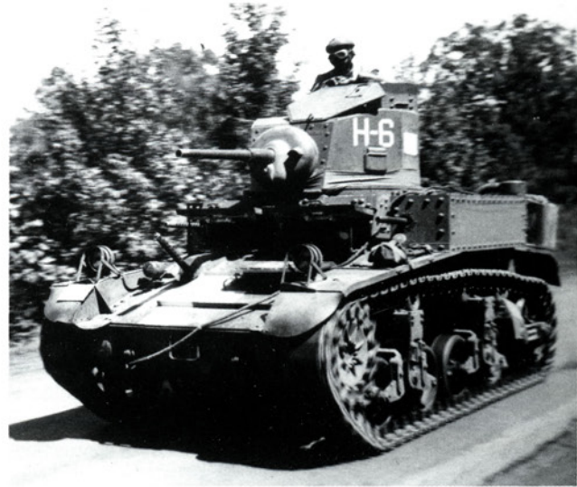
Above: An M2A4 light tank at Fort Benning in 1941. Note the sponson-mounted .30-cal machine guns, riveted construction and early-style tank's helmet. Courtesy of Mark Bando
